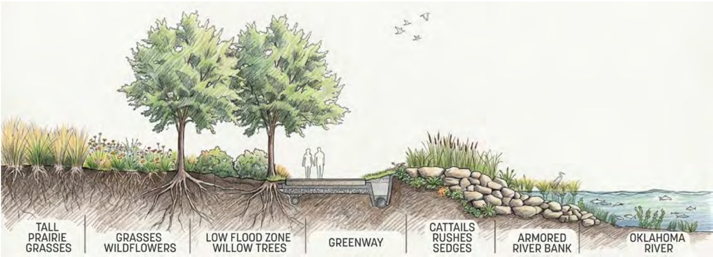
Proposed ecologically enhanced cross section for riverfront.
